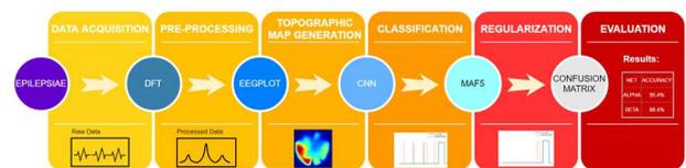
Figure 1: Processing pipeline of the DM process
