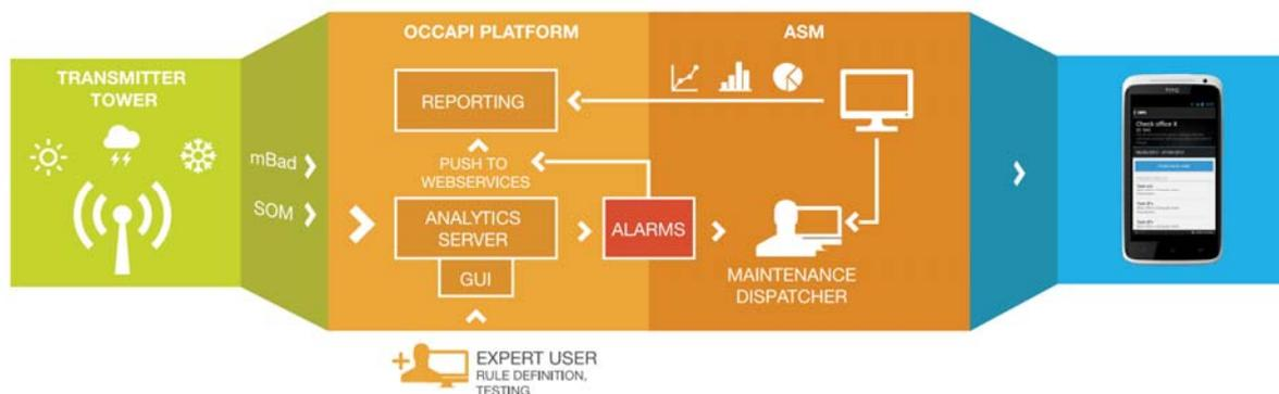
Figure 3: Architecture of the ASM OpComm solution.
