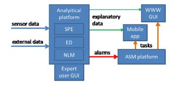
Figure 1: Proposed conceptual architecture for event processing in asset management use case. SPE represents Stream Processing Engine, ED Event Detection and NLM Natural Language Module.
